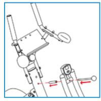
Insert the front bolt (C) to attached the bow-rail to the main structure in order to perform the AB FRONT exercise
